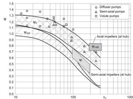
Fig. 2 Pressure coefficients
