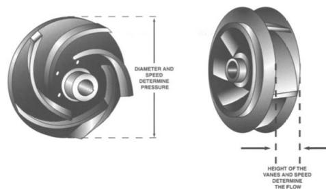
Fig.1 Pump Impeller
