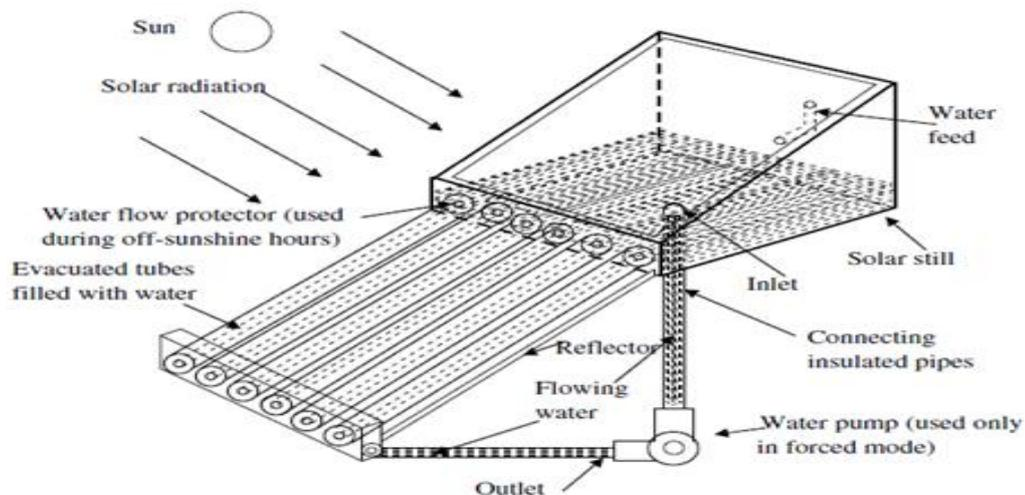
Fig. 9 Schematic of Evacuated glass tube Integrated Solar Still in forced circulation mode [20]
