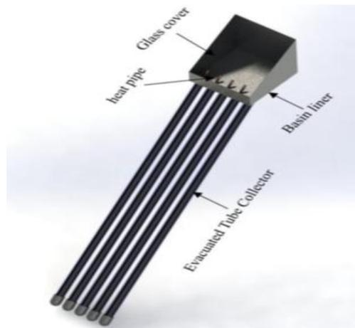
Fig. 5 Proposed model of solar still coupled with ETC with thermosiphon heat pipe [14]
